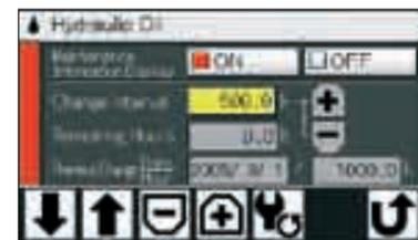
Replacement timing of hydraulic oil and fuel filters is alerted to the operator through the LCD monitor according to the schedule preset by the user each time when turning the key switch. The scheduled maintenance can prevent the failure of the machine.
