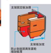
⑤坚固的D型断面封闭式机架
