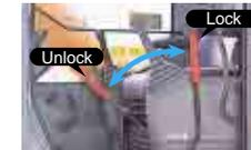
Pilot-control shut-off lever
