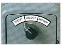
Extra Port that Sets Optimum Flow to Optional Attachment: The extra port is a hydraulic source for setting and delivering the optimum oil flow to optional attachment that is well matched with the front attachment.
