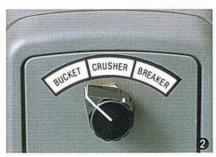
Extra Port that Sets Optimum Flow to Optional Attachment: The extra port is a hydraulic source for setting and delivering the optimum oil flow to optional attachment that is well matched with the front attachment. Attachment Mode Optionally Available: The attachment mode can be selected with the attachment selection switch according to the attachment used. This makes combined opera-
